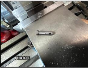
Four 2-inch-long reach clevises were made for 3/8-inch square stock. I used the same method for finding the center of the stock to mill the 3/16-inch opening 1.375-inch along the center. To make the round end of the clevis I happened to have a 3/8-inch square collet.
