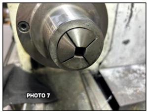
Photos 7,8 and 9. The milled clevis were put in the collet and turned the material and drilled for the 10-32 left had tap. A short 3/8-inch hex piece is silver soldered on the brake rods to make adjustments easier.
