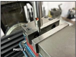
The edge finder has a .02-inch diameter round contact. Once the finder touches the edge for the vice, I raised the quill and moved the table .01 inch, inward and now have the starting point for locating the center of the material. In this case moving the table along the y axis .187 inches. Photo 4.
