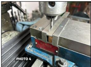
After all the holes were drilled, I made the .187-inch diameter pins. To keep the pins in place 1/16-inch cotter pins are used. To drill a hole for the cotter pins that is through the center of the pin I made a fixture to drill the holes. Photos 5 and 6.
