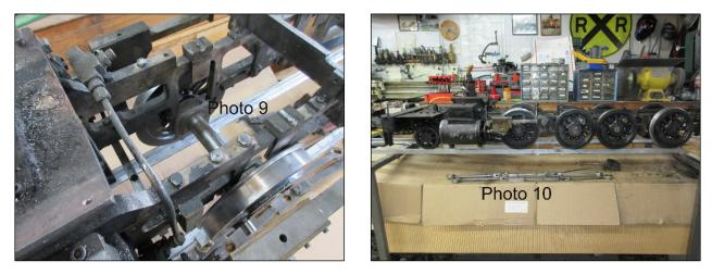
Next items: Install the brakes, install the side rods and check to see if any of the bronze bearings need replacement and finally install all the valve gear and set the timing.
