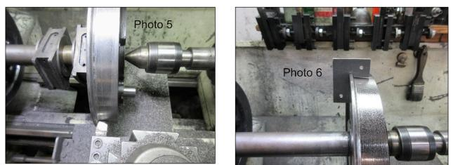
inch gauging radius. Photo 5 shows the tool being used to machine the flanges of the first and fourth set of drivers.
