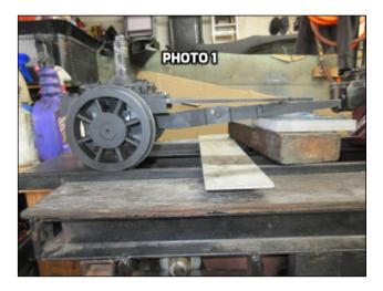
The parts I was having trouble with were the transverse bar, the equalizing bar and the pivot base for the transverse bar. After reading the chapter and studying the drawing, I proceed to make some modifications to the truck to get it properly installed and functional. This process took about two weeks. Photo 2 show the installed truck. Arrows show the changes. Orange: Equalizer bar, Yellow: Transverse bar.
