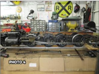
Next is installing the valve gear and setting the timing. Very soon, I hope to have the C16 chassis back to RLS.
