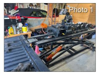
chassis on to the back of my pickup. I made the stand, which has a 8 ton hydraulic jack that can raise the top rails to a height of 40 inches.
