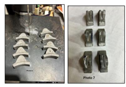
I then cut the wheel on a band saw which gave me eight separate brake shoes. Photo 6.
