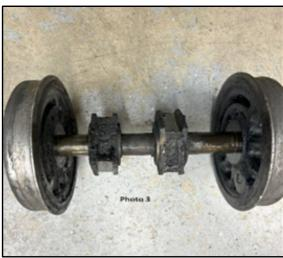
from the axle, I can inspect the journal boxes to determine if it is possible to insert needle bearing. Photo 2 shows the drivers. Photo 3 shows the journal boxes, which are free to move on the axles. Since I did not have the fixture to remove the axles, I decided to work on the brakes.
