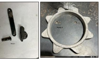
Steamers had freight wheels, brake shoes, freight journal boxes and truck side frames cast in Tijuana. I have an extra set of brake shoes which I will use for this project. Photo 5 shows the shoes which are cast in aluminum.
