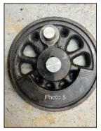
With one of the wheels removed, I made two pins (one for axle bore and one for the crank pin bore) to measure the crank pin throw. The measurement is 2.0625-inches. *Photo* 5
