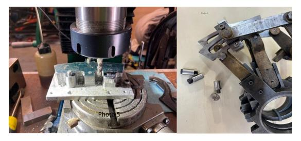
I made two sets of links block, one set was just like the original set, that is slotted. I made another set that can be easily replaced with an Allen screw. The original link blocks were round rather than square. I decided to keep with round blocks. Photo 6 shows the complete valve gear with the link blocks.
