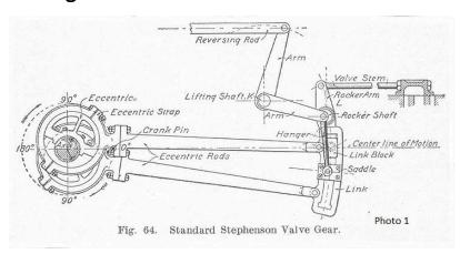
After removing the valve links, measurements were taken to determine the amount of wear. The original width of the link, where the link block travels was .4375. The bottom of the link was .448 and the top of the link was .475. The blocks were very worn.
