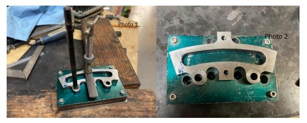
The new links are made from 5/16 tool steel, which I later hardened. I put the two blanks together, so that both links would be the same. After removing the excess material on the band saw, I used a jig I had made for machining the links for my ten-wheeler, to make all the radius cuts on the mill. The link slot for the link blocks is an 8-inch radius. Photo 3 and 4
