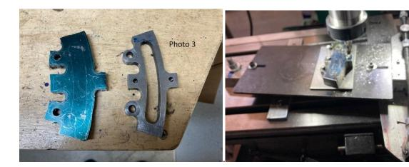
To get the round sections where the pins go that connect to the eccentric rods, I use a rotary table to mill the round sections Photo 5.
