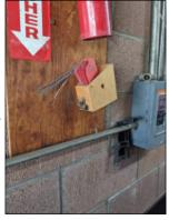
Take a service tag, fill out the top and bottom, tear off the bottom and stick that into the clip holder on the box then attach the tag to the bad order car so that it can be clearly seen by other members or myself (attaching on or near the coupler works great).
