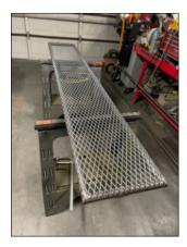
Tom has started welding up steel expanded metal benches. These new benches will be powder coated and will match the design of benches used throughout the park.
