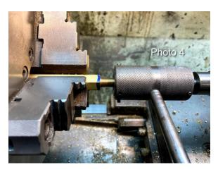
**Photo 4** show tapping the end of the bonnet ¼-40 thread to the bonnet cap. Which I made from 5/16-inch brass hex stock.
