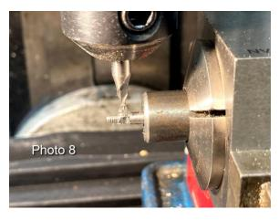
**Photo 8** show machining the square part of the stem just below the 2-56 thread. The milling cutter is 3/32. One side is machined, the block is turned a quarter turn, the next side is machined and so on.
