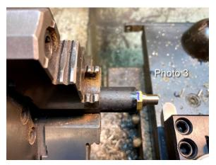
**Photo 3** show the upper part of the bonnet being shaped. I have a 3/8-inch-high speed tool bit that has been ground with a 3/8 diameter inch round end.
