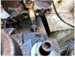
The wheel is then parted off at 3/23 inch thick.
