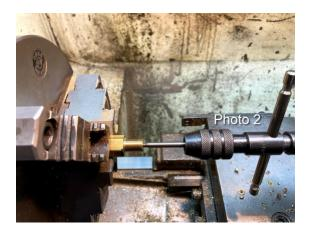
**Photo 2** show taping the inside the of bonnet for 8-32 thread. I used 9/16-inch brass hex stock to make the bonnet. The screw size that goes into the valve body is 3/8-32. The stem that goes into the bonnet has three sizes.
