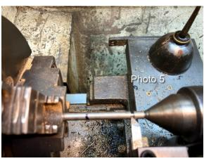
The stem is 1 5/8 inches long. I use a very sharp high-speed tool, using .010 depth of cuts. First the rod was turned down to .187. Then it was turned down to the major diameter for the 8-32 thread (.164) for a length of 1.22 inches. Then it was turned down to .123 inches for .95 inches. For this part I use only depth of cuts of .005 inches.
