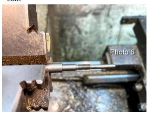
**Photo 6** shows the stem after the machinating is complete and the part is ready to be cut off.
