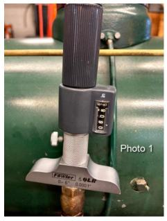
In **Photo 1** the distance from the top of the ball to the top of the valve body is .603 inches. Subtracting that from the ball travel amount I need to make the part of the bonnet that screws into the valve body .52 inches.
