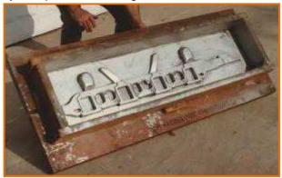
ductile iron, or non-ferrous material such as bronze. It can be done of course but it can lead to increased casting costs due to the possible "creative gating" and risers which could be encountered when casting steel. I didn't need something to increase the cost unless there was a good solid reason for doing so, a principal that my supervisor at work pounded into my head
