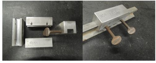
Procure some ¼" X 20 X 1" long THUMBSCREWS & grind ends flat and polish so Aluminum rail edges do not get buggered up. Some may be concerned about the cast iron wheel flange bumping into the chock so they may want to machine a notch in all 4 ends of the chocks so the tread contacts the chock instead of the thin flange.
